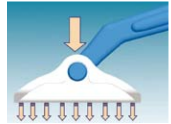
Unique blade design transfers scraping force to the blade edge, allowing it to conform to the scraping surface.
