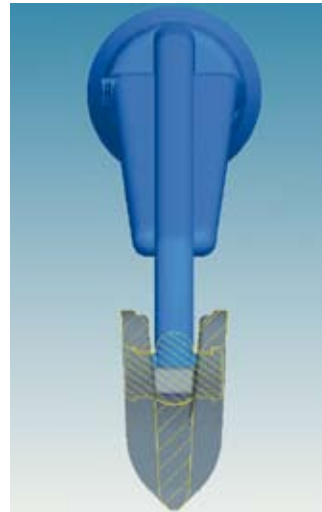
Larger handle diameter for better gripping. Sharper scraping edge and more compliant blade material.
