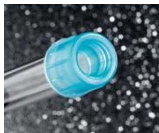
Sterile tube (12 x 75 mm) with cell-strainer cap Designed for flow cytometry applications, the 12 x 75 mm tube with cell strainer cap (Cat. No. 352235) offers a convenient way to prepare laboratory samples. A 35 µm nylon mesh is incorporated into the tube cap, which can be used to collect the dissociated sample for downstream processing in instruments such as the BD FACS™ System.
