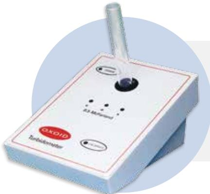
A turbidometer, for the accurate preparation of 0.5 McFarland inoculums, is also available, aiding standardization and contributing to reproducible, reliable results. The turbidometer is simple to use, giving clear indication of the density of the inoculum.
